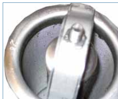
Filter cleaned in an ultrasonic bath
