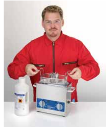
Drill head cleaning in the ultrasonic cleaning unit RK 102 H
